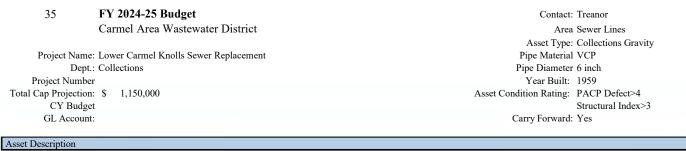
Replace approximately 3160 linear feet of existing 6-inch clay pipe with a new 8-inch High-Density Polyethylene (HDPE) and includes manhole rehabilitation
