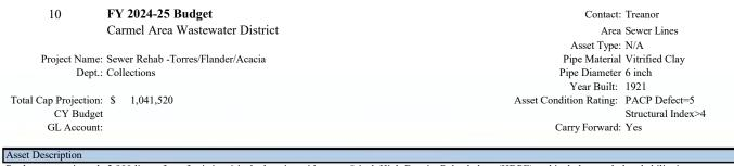
Replace approximately 2,900 linear feet of existing 6-inch clay pipe with a new 8-inch High-Density Polyethylene (HDPE) and includes manhole rehabilitation
