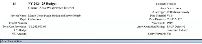
Replace approximately 4,376 linear feet of existing 6, 10 and 12-inch clay pipe with a new High-Density Polyethylene (HDPE). Includes manhole rehabilitation. Replace and repair portions of pump station as needed.
