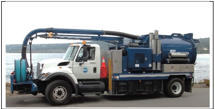
Photo: CAWD Vactor Truck
