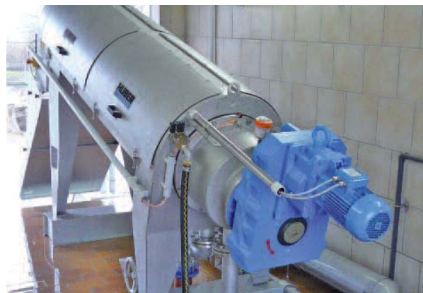
Screw press for 24/7 unattended operation
