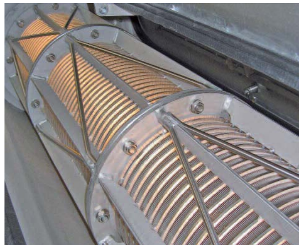
Sturdy screen basket made of stainless steel
