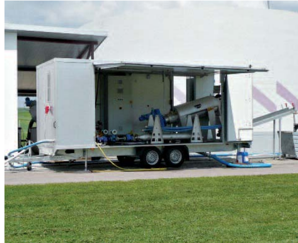
Mobile screw press in a trailer
