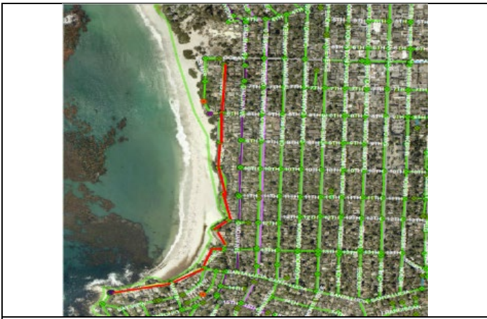
Photo: Pipe Bursting Limits on Scenic
